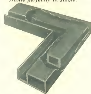
The illustration above gives some idea how the fine mesh screen cloth is held so tightly in place. The "cloth" is first rolled into the groove. When the spline is inserted it draws cloth taut and holds it firmly. The spline is easily removed should wire cloth become damaged and need replacing. The cut away corner shows the heavy reinforcing in the corner of Higgin All Metal Screens. These rigid angles hold the frame perfectly in shape.
